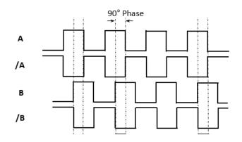
In the table above the cable colors of sensors output signals are given. If the control circuit is suitable in the Line Driver sensors of the not output signals (/A, /B) have to be added to the system. If it is not suitable /A, /B signal cables must be fixed as insulated separately. Don't forget that these edges have electricity too.
