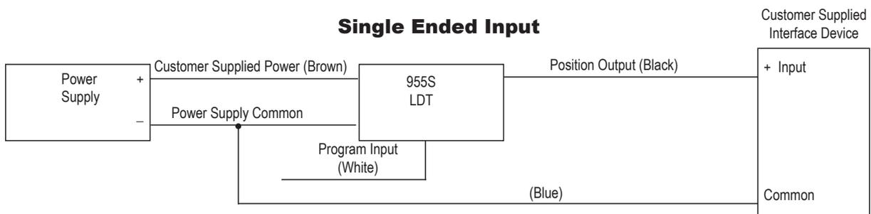
NOTE: 955S-C is current sourcing, which allows the current to flow from the LDT into the user's equipment.
