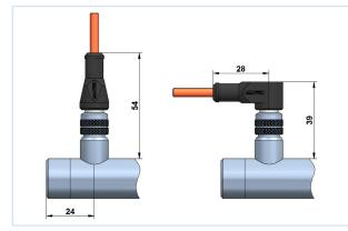
For sensors with connector output the cable has to be ordered separately. You can choose from a cable with a straight connector or with an angular connector.
