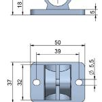
Fußklemmstück 20-VA, base clamp material: stainless steel, temperature resistant up to 200 °C
