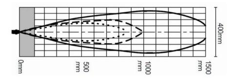
The cone size is set by connecting the teach input for >5 s with the power supply  $-U_B$  (0V). See also the teach table at page 4:
