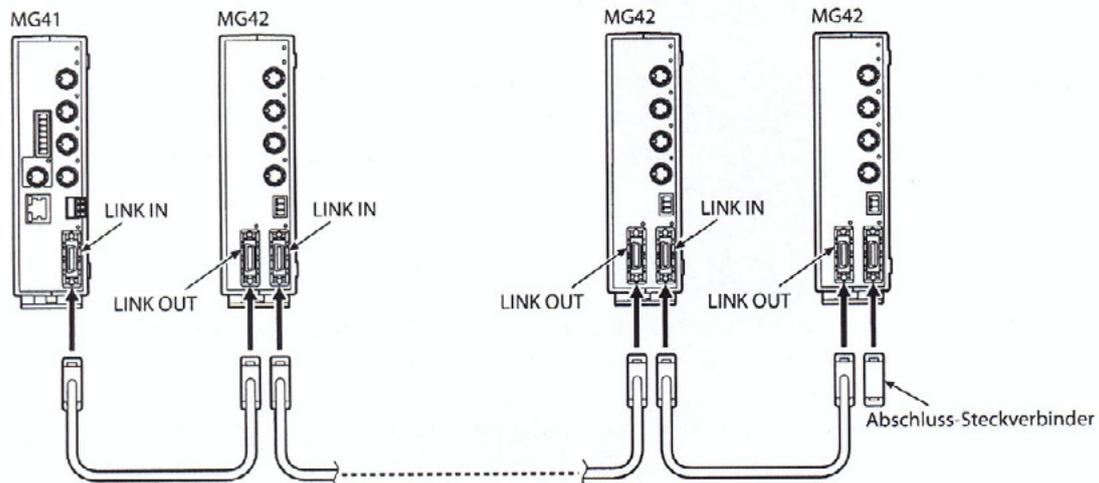
**Note:** Do not remove the link cable while the power is on. Disconnecting the cable will cause a communication error and the system will have to be restarted.
