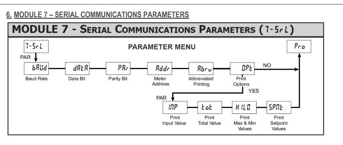
It is necessary to match the PAX meter's serial communications parameters to the host's parameters before communications can be established. This is accomplished by using the PAX front panel keys to enter **7-5-L**.
