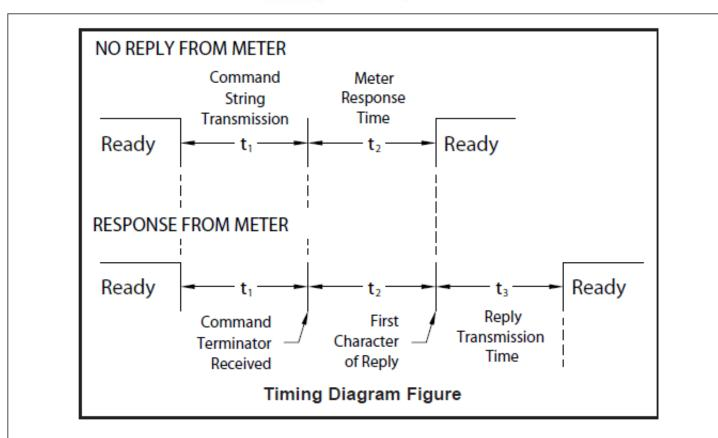
At the start of the time interval  $t_1$ , the computer program prints or writes the string to the com port, thus initiating a transmission. During  $t_1$ , the command characters are under transmission and at the end of this period, the command terminating character (\*) is received by the meter. The time duration of  $t_1$  is dependent on the number of characters and baud rate of the channel.
