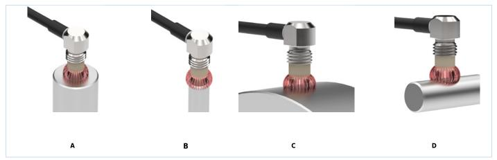
A Optimum object surface preferably 2-3 times greater than the probe head diameter. The sensing field is captured by the object entirely.
