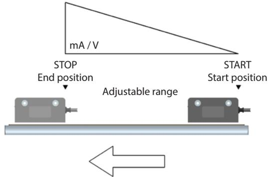
With ascending ramp, before the initial position of the travel the encoder will provide the minimum current / voltage signal level of the output range (4 mA for AI1; 0 V for AV2). After the last position of the travel the encoder will provide the maximum current / voltage signal level of the output range (20 mA for AI1; 10 V for AV2).
