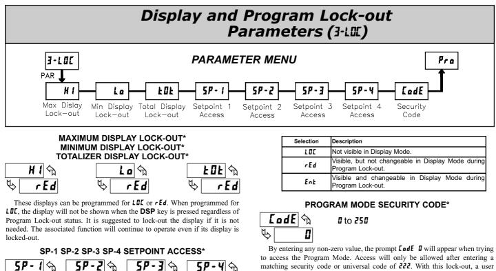
The setpoint displays can be programmed for LOL, rEd or Enk (See following table). Accessible only with the Setpoint plug-in card installed.
