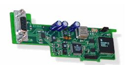
The PAX PROFIBUS-DP Communications Option Card provides a direct connection for a PAX panel meter to a PROFIBUS-DP Network. This allows a PROFIBUS Master device, such as a PLC, to control and monitor the operation of the PAX meter. The meter functions as an intelligent PROFIBUS-DP Slave device on the Network.
