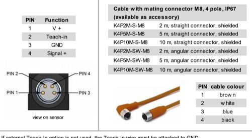
If external Teach-In option is not used, the Teach-In wire must be attached to GND.
