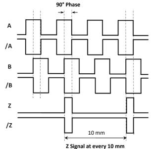
In the above table, the cable colors of sensors output signals are given. If the control circuit is suitable in the Line Driver, sensors of the not output signals (/A, /B, /Z) have to be added to the system. If it is not suitable /A, /B, /Z signal cables must be fixed as insulated separately. Don't forget that these edges have electricity too.
