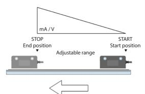
With ascending ramp, before the initial position of the travel the encoder will provide the minimum current / voltage signal level of the output range (4 mA for Al1; 0 V for AV2). After the last position of the travel the encoder will provide the maximum current / voltage signal level of the output range (20 mA for Al1; 10 V for AV2).
