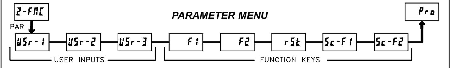
The three user inputs are individually programmable to perform specific meter control functions. While in the Display Mode or Program Mode, the function is executed the instant the user input transitions to the active state.
