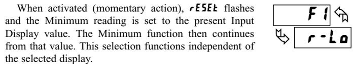
When activated (momentary action), rESEt flashes and the Minimum reading is set to the present Input Display value. The Minimum function then continues from that value. This selection functions independent of the selected display.
